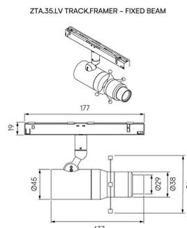
Modular high-performance, low voltage track-mounted spotlight system, for interior architectural applications such as Museums, Galleries, Retail and Workplace environments. Engineered for exceptional durability, maintainability, re-manufacturability, and recyclability, this spotlight sets a new standard for sustainable design.
