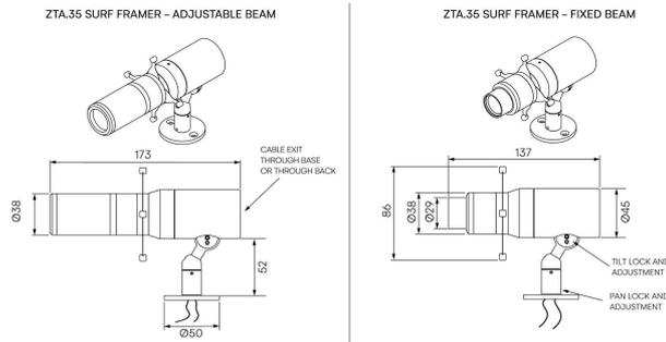
Modular high-performance, surface mounted spotlight system, for interior architectural applications such as Museums, Galleries, Retail and Workplace environments. Engineered for exceptional durability, maintainability, re-manufacturability, and recyclability, this spotlight sets a new standard for sustainable design.
