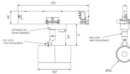
Modular high-performance, mains track-mounted spotlight system, for interior architectural applications such as Museums, Galleries, Retail and Workplace environments. Engineered for exceptional durability, maintainability, re-manufacturability, and recyclability, this spotlight sets a new standard for sustainable design.
