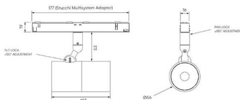
Modular high-performance, low voltage track-mounted spotlight system, for interior architectural applications such as Museums, Galleries, Retail and Workplace environments
