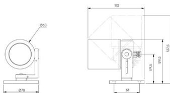
High-performance exterior spotlight system, for surface mounting to illuminate exterior architectural details and landscape illumination.
