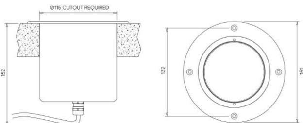
Exterior in-ground recessed adjustable and lockable uplighter, for enhancing architectural details, gardens and pathways.
