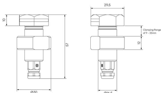
Miniature exterior semi-recessed marker light, providing soft and low levels of light for pathways to assist with wayfinding.
