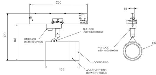
Modular high-performance, mains track-mounted spotlight system, for interior architectural applications such as Museums, Galleries, Retail and Workplace environments. Engineered for exceptional durability, maintainability, re-manufacturability, and recyclability, this spotlight sets a new standard for sustainable design.
