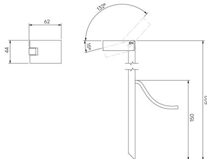
Low level exterior rated adjustable spike light, providing soft and wide light distribution for pathways.
