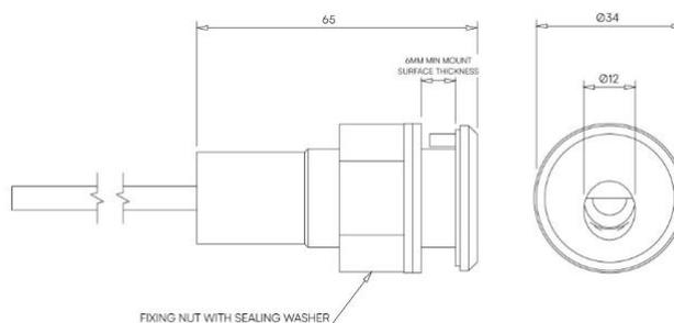
Exterior recessed wall light, for enhancing pathways, stairs and decks.
