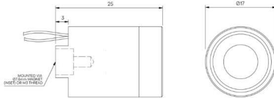
Miniature recessed fixed focus module, for enhancing both interior and exterior architectural details. Capable of recessing into walls, ceilings and furniture.
