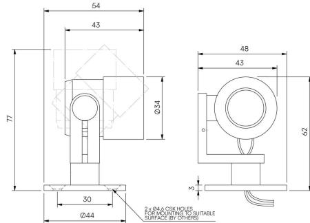
High-performance exterior spotlight system, for surface mounting to illuminate exterior architectural details and landscape illumination.
