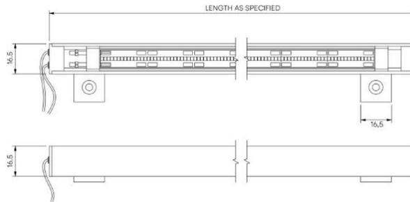
Linear lighting system, typically for under seat, planter and handrail lighting applications.
