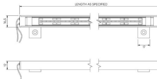
Linear lighting system, typically for accent lighting and integration into interior architectural details.
