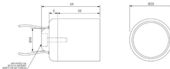
Compact recessed fixed focus module, for enhancing both interior and exterior architectural details. Capable of recessing into walls, ceilings and furniture.
