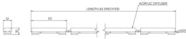
Flexible, modular linear lighting system for cove and handrail lighting applications.
