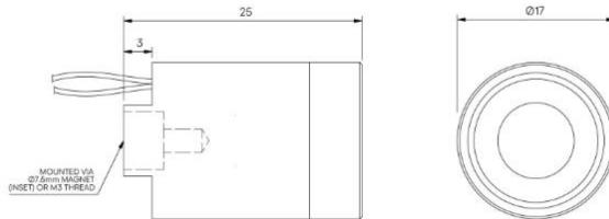
Miniature recessed fixed focus module, for enhancing both interior and exterior architectural details. Capable of recessing into walls, ceilings and furniture.
