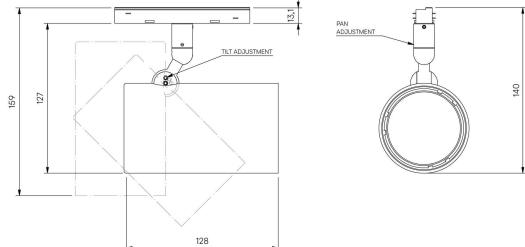
Modular high-performance, low voltage track-mounted spotlight system, for interior architectural applications such as Museums, Galleries, Retail and Workplace environments. Engineered for exceptional durability, maintainability, re-manufacturability, and recyclability, this spotlight sets a new standard for sustainable design.
