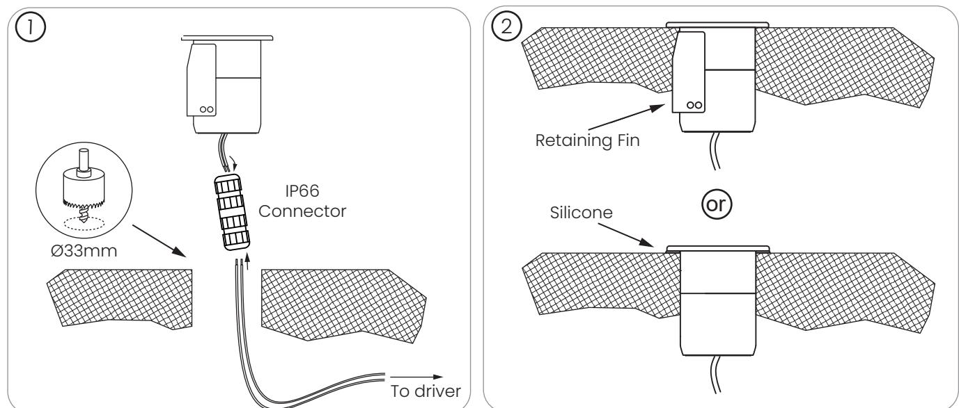
Surface gradient must run away from the fitting.
