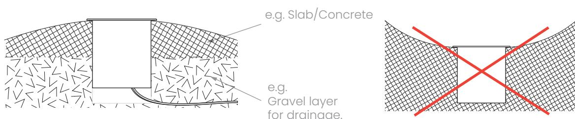
If installing in solid ground, additional drainage must be provided (e.g. a bed of gravel as shown).
