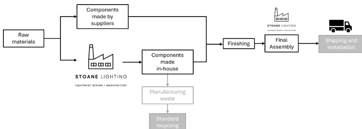
Figure 1: Scheme representing the main steps involved in the sourcing and manufacturing processes before the product is ready to be shipped to the customer.
