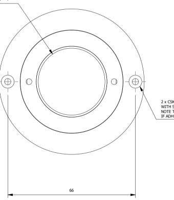
2 x CSK HOLES FOR MOUNTING WITH SUITABLE FIXINGS.
